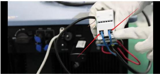
2. Connect one end of the communication cable to the meter. (PIN 4,5 of the communication cable to PIN 5, 6 port of the meter).
