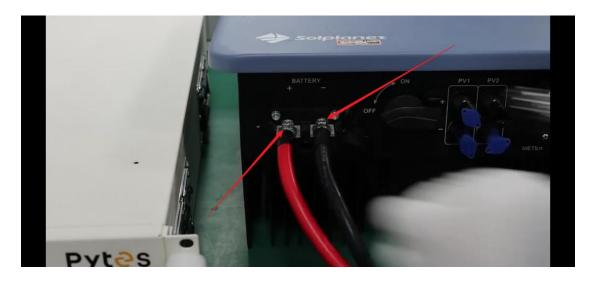
4. Double-check to ensure that the positive terminal of the battery is connected to the positive terminal of the inverter, and the negative terminal of the battery is connected to the negative terminal of the inverter.
