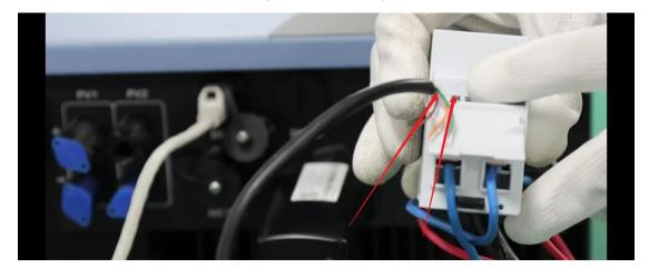
3. Connect the opposite end of the communication cable (RJ45) to the meter port of the inverter.
