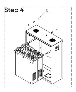
Place and fix the batteries in cabinet with screws.
