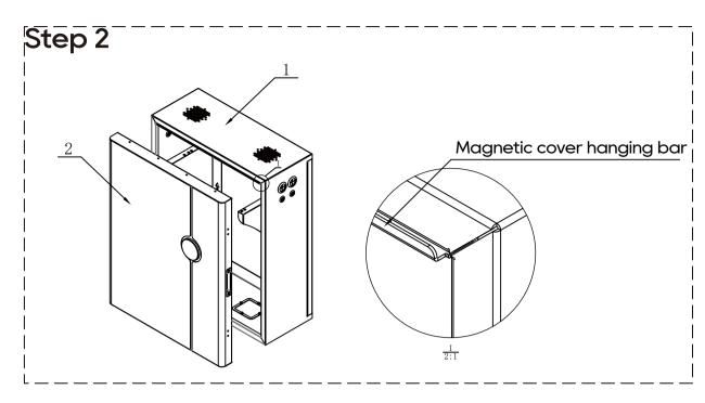
Lift upwards and pull it to remove the magnetic cover from main cabinet.
