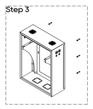
Install the main cabinet to wall by securing to the expansion screws.
