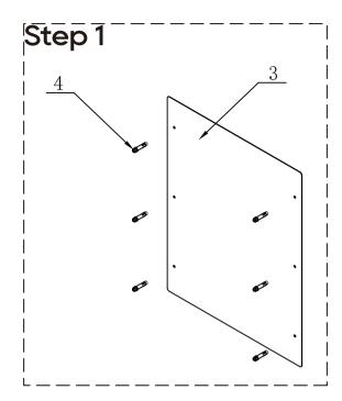
Use positioning board to determine installation position of the cabinet. Drill and install the expansion screws.
