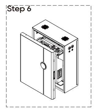
Align the sides of magnetic cover to main cabinet then place downwards.
