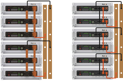
Figure 5-1 Schematic diagram of power cable connection
